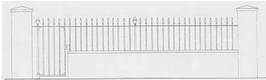
***Typical elevation of domestic iron railings with brick piers on either side and brick dwarf wall.***
