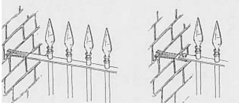
**Example of fixing where the fish-tail end of the top rail can be built into the brickwork.**
